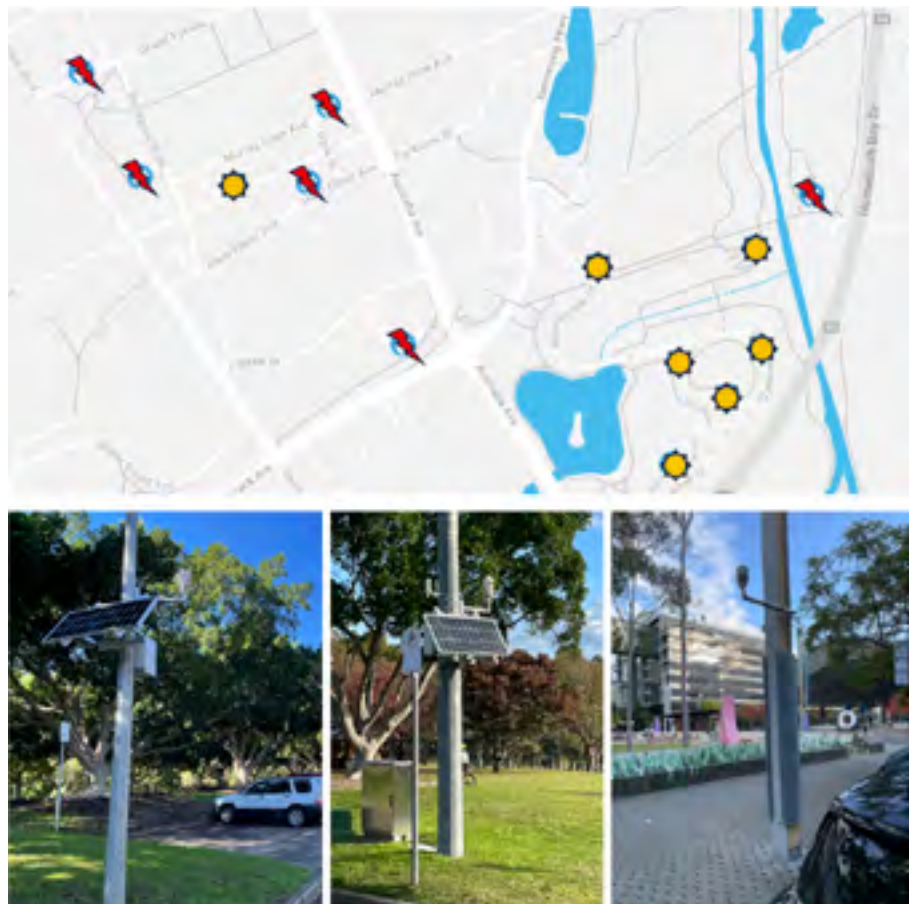
Figure 3: Geographic location and exemplary images of the thirteen weather stations used during Phase 2. Lightning symbols denote weather stations with permanent power, sun symbols indicate solar panel-powered stations. Images show stations: left - 1 (Village Green), middle - 4 (north of Waterview building), right - 11 (Abattoir Blues Corner).
